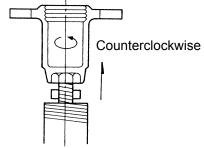
Loosen the locknut
