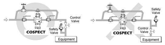
When installing a safety valve to protect the air equipment, be sure to install it on the air equipment or directly before the inlet of the air equipment. If the safety valve is installed on the outlet side of the **COSPECT** between the **COSPECT** and a control valve, an eventual pressure rise could activate the safety valve.
